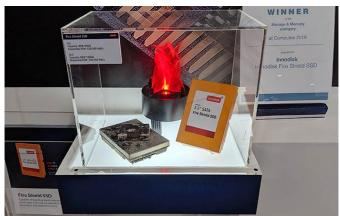
Featuring heat proofing technology patented by the USPTO, the Fire Shield SSD features three layers of protection. The first enclosure consists of a flame-resistant copper alloy material, while the second uses a heat-isolating lining material. A third protective enclosure houses the actual SSD. Innodisk says the design uses over 20 heat-resistant materials, and it ensures the SSD is not only fireproof, but also vibration- and impact-proof.
