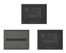
The 256GGb V-NAND offers energy efficiency comparable to the 64-layer predecessor, since operating voltage is down from 1.8V to 1.2V. Meanwhile data write speed reaches 500 microseconds, a 30% improvement over the previous generation, and response time to read-signals is reduced to 50 microseconds. Inside the chip are 90 layers of "3D charge trap flash" (CTF) cells, stacked in a pyramid structure with microscopic channel holes vertically drilled throughout.
