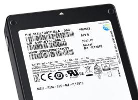
Aimed for enterprise systems, the PM1643 doubles the capacity of the previous 15.36TB Samsung SSD through the combination of 32 new 1TB NAND flash packages. Each package is comprised of 16 stacked layers of 512Gb V-NAND chips, and allows the storage of approximately 5700 5GB HD movie files in a 2.5-inch device.
