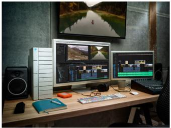
According to the company, such speeds come through the combination of the hardware RAID controller, 256MB cache and 7200RPM Seagate enterprise-class drives. This makes the drives ideal for photography professionals moving large amounts of RAW footage from a Blackmagic camera to a Adobe Premiere, before editing multiple ProRes 422 (HQ), ProRes 444 XQ and even uncompressed HD 10-bit and 12-bit video streams.
