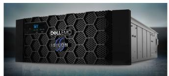
According to the company Isilon All-Flash combines the performance of flash technology with the scalability, multi-protocol access and security of the Isilon OneFS OS. It features a dense blade-node architecture consisting of 4 Isilon nodes within a singe 4U chassis, with capacity options ranging from 92 to 924TB per chassis.
