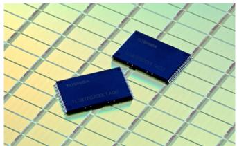
Western Digital (WD) presents the next generation of 3D NAND flash-- BiCS3, featuring 64 layers of vertical storage capability on a single 3-bits-per-cell chip, making it the smallest from the company.
