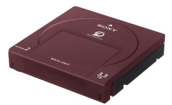
The companies claim the optical media offers a 10-year shelf life while doubling single cartridge capacity to 3.3TB. The 2nd generation Optical Disc Archive cartridge also features an 8-channel optical drive unit offering twice the read/write speeds over the previous generation, allowing it to handle real-time 4K video playback.
