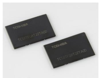
BiCS flash uses a 48-layer stacking process to surpass the storage capacity of current 2D NAND flash while enhancing write/erase reliability, endurance and write speeds. Back in March Toshiba revealed an earlier version of the technology with 128 gigabit (16GB) 48-layer BiCS non-volatile memory chips.
