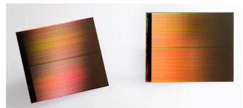
The result of over a decade of R&D, 3D XPoint memory features a transistor-less cross point architecture built in a "3D checkerboard." Memory cells sit at the intersection of word lines and bit lines, allowing the individual addressing of cells. The result is data written and read in small sizes, leading to faster and more efficient read/write processes.
