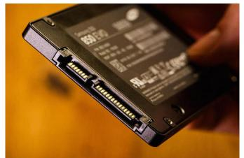
According to the study, the period of time "some" SSDs retain data when unpowered can be slashed in half for every 5°C rise in ambient temperature. In other words, if an SSD retains data for 2 years if kept at 25°C, that length of time is cut down by half (to 1 year) if the temperature rises to 30°C.
