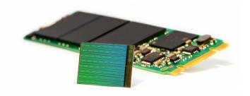
According to the two company 3D NAND allows for three times higher capacity than competing NAND technologies while keeping flash storage performance gains and cost savings aligned with Moore's Law.
