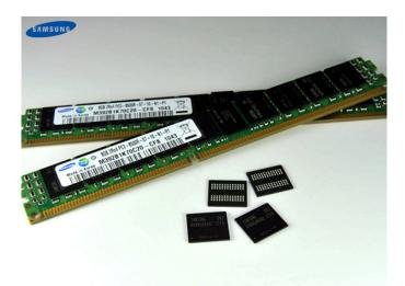
The new registered or buffered (RDIMM) product is based on Samsung's own Green DDR3 DRAM and 40nm circuitry.
