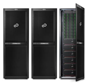
The CD10000 is based on Ceph, the open source storage software from Red Hat-owned Intank. It presents a unified view of block, object and file storage in a single distributed storage cluster, and theoretically allows for scaling to up to 1 exabyte. This means it does not use RAID, and protection comes from replication and the system self-heals with zero downtime, at least according to Fujitsu.
