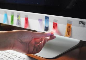
Currently still in the concept stage, the dataSTICKIES would stack on top of each other like a pack of post-it notes. The idea goes that one simply "peel" a drive from the stack and stick it (via low-tack multiuse conductive adhesive) to a proprietary wireless interface, the so-called Optical Data Transfer Surface (ODTS), in order to transfer data.
