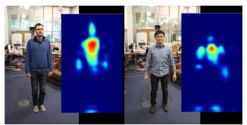
Dubbed RF-Capture, the technology uses variations in wifi signals to recognise human silhouettes from behind walls. To do so it first transmits wifi signals before analysing reflections in the signals to piece together a human form. In other words, it is a little bit like a radar. It requires no wearable sensors and transmission power is "10000 times lower" than standard mobile phone signals.
